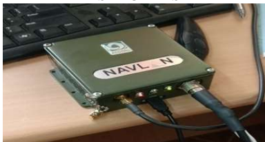
Single frequency GNSS/SBAS Receiver
