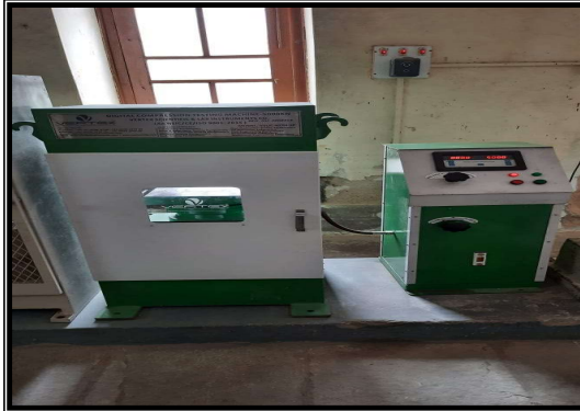
Compression Testing Machine Capacity: 5000 KN
