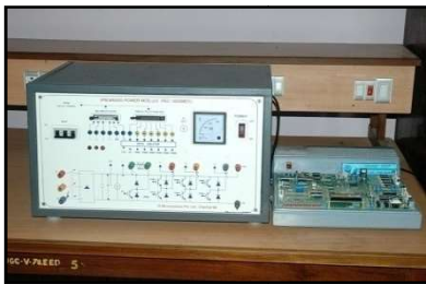
IPM Power Module with DSP Controller
