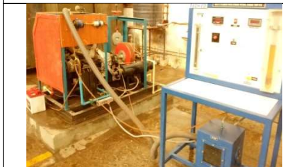
Multi cylinder 4 stroke petrol engine test rig
