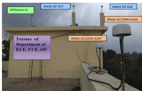
GNSS Antenna's Setup for Real-time Data Acquisition(AGRL)
