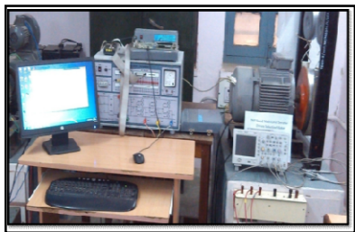
DSP based Multilevel Inverter Fed Induction Motor Drive
