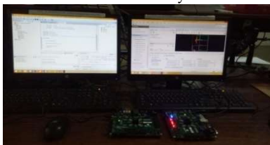
ZedBoard Zynq-7000 ARM/FPGA SoC
