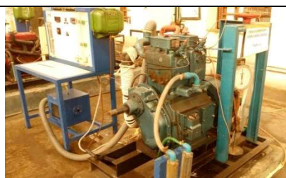
Twin cylinder 4 stroke diesel engine test rig
