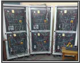
Feeder Protection Unit (Power system Lab)
