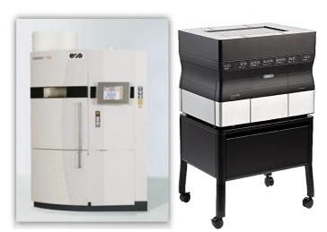
EOS SLS Rapid Prototyping SystemSTRATASYS Polyjet 3D Printer
